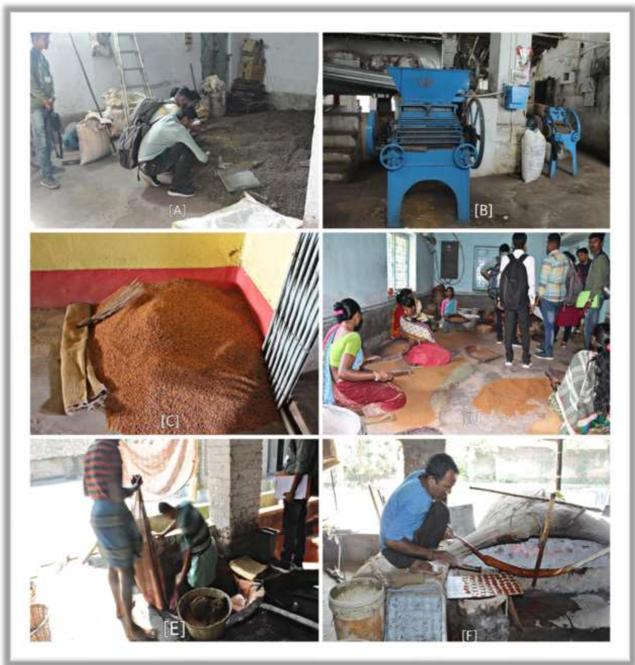
Plate 1.2: Photographic evidences of industrial processes in lac factories (A) Raw lac (B) Crushing machine (C) Washed lac (D) Sieving of lac in different granular sizes (E) Washing of lac in cement pot (F) Melting of lac in coal oven.
