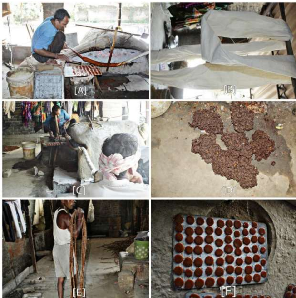
Plate 1.3: (A) Preparing of lac button (B) Cotton cloth used to melting lac (C) Preparation of lac melting (D) Inferior products or by-products of lac (E) Drying of cotton cloth (F) Final product of lac button.
