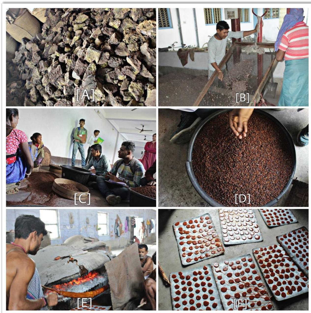
Plate 1.4: Photographic evidences of (A) Crude Lac (B) Sieving by male workers (C) Sieving by female workers (D) Seed Lac (E) Melting of lac in oven (F) Prepared Lac button.
